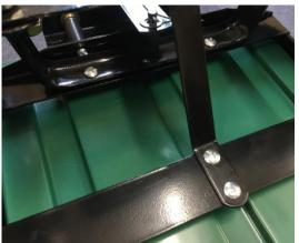
3. Attach the Front axle support with braces (F) to the frame (B) using 4 small bolts (I) and 4 small bolt washers (J).
