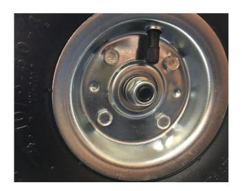
Attach the 4 wheels (H) to each axle bar, and secure this by using 4 gaskets (L) and the large locking nut (K).
